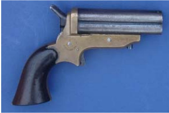
USA, Sharps 4 barrel Derringer, 1862, 4 shot, single action equivalent, .22 or .32 cal, barrels slide forward to load
