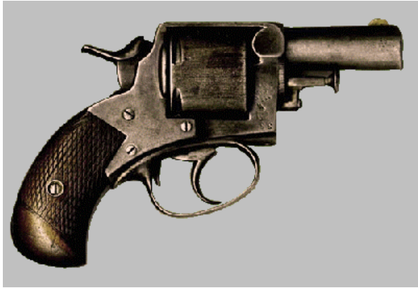
England, Webley Bulldog revolver, 1878, double action, 6 shot, .38 or .442 cal, 2.5" barrel
