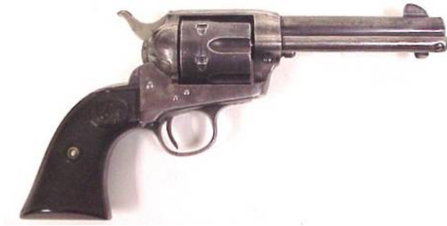
USA, Colt Army (Peacemaker) Revolver, 1873, single action, 6 shot, .45 cal (and various other calibers), 4 3/4" barrel, also 3", 5 1/2" and 7 1/2" round barrels are standard but barrel lengths were from 2" to 16"
