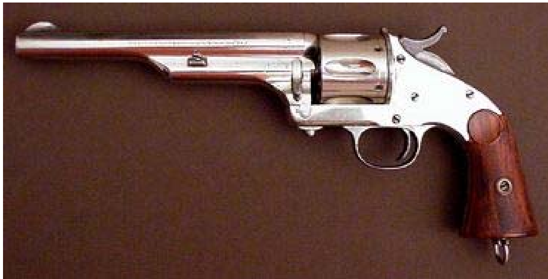
USA, Merwin Hulbert Frontier Revolver, 1876-77, single action or double action, 6 shot, .38 or .44 cal, 6" or 7" round barrel, lanyard ring
