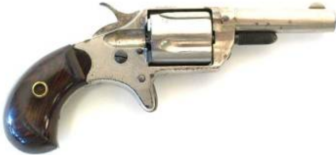
USA, Colt New Line Revolver, 1874-1876, single action, 5 shot, .22 and .30 short and long cal RF, 1 3/4" or 2 1/4" round barrel, the longer barrel was standard
