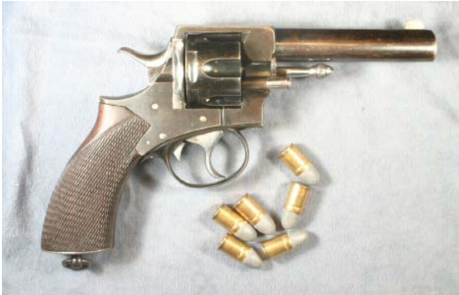
England, Webley RIC Revolver, 1868, double action, 6 shot, .442 cal, 4.5" barrel
