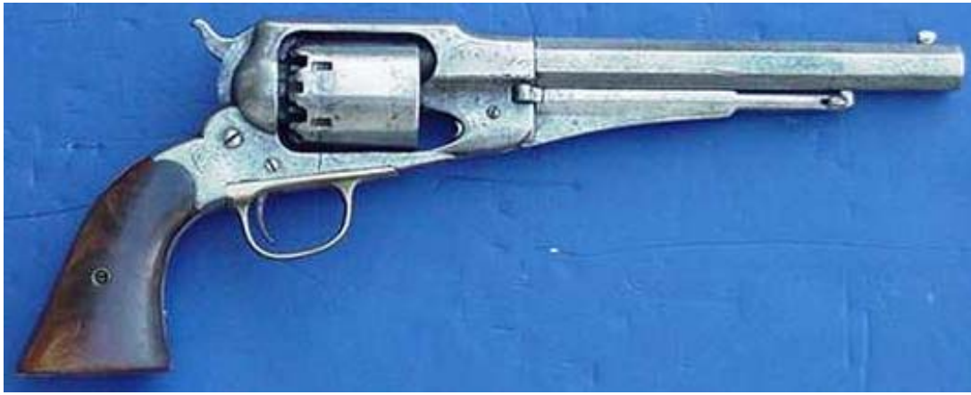
USA, Remington Army Mod. 1861 Percussion Revolver, 1861, single action, 6 shot, .44 cal
