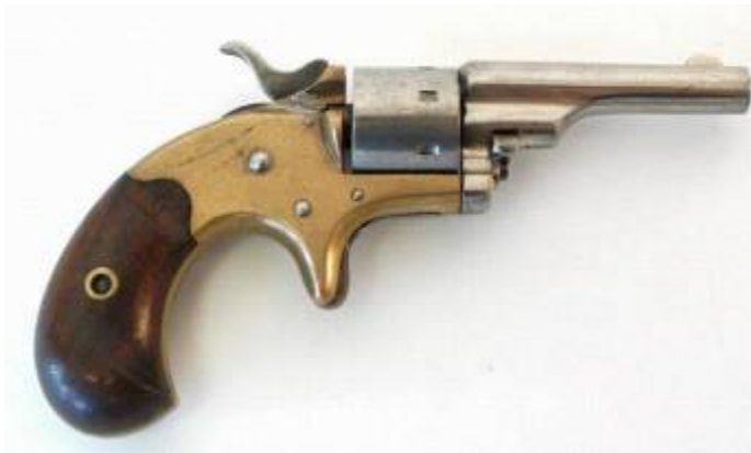
USA, Colt Open Top Pocket Revolver, "Old Line", 1871-1877, single action, 7 shot, .22 cal short and long RF, 2 3/8" or 2 7/8" round barrel
