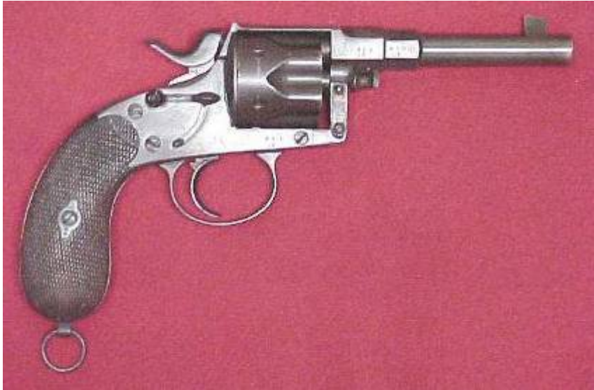
German, Reichs Revolver, 1883, double action, 6 shot, 10.6 mm, lanyard ring
