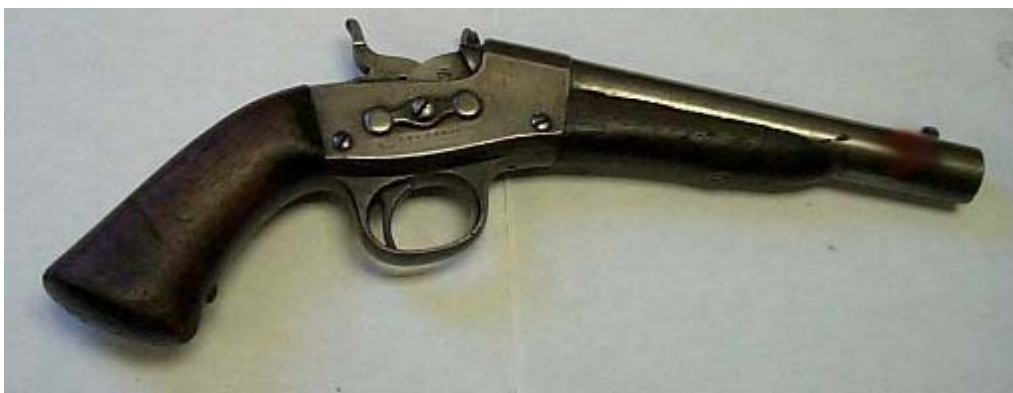
USA, Remington Navy Rolling Block Pistol, 1867, single shot, .50 cal CF
