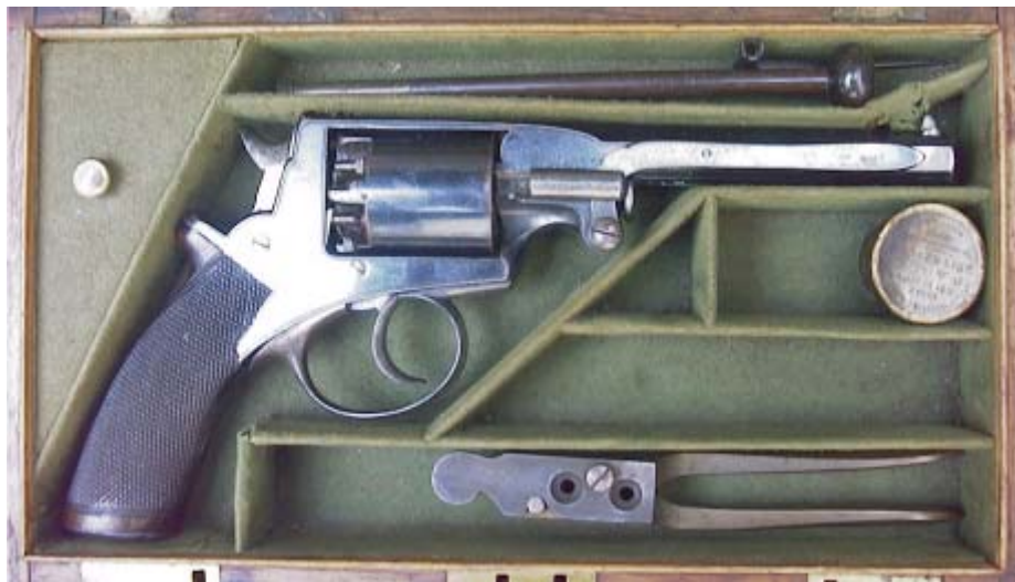
England, Adams percussion Revolver, 1851, double action, 5 shot, .32, .44, .45 cal, 5" barrel
