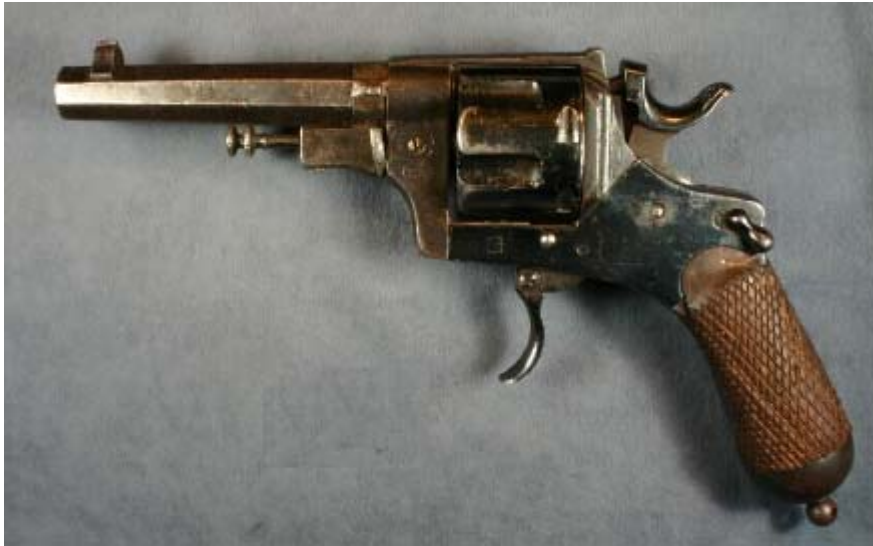
Italy, Bodeo revolver, 1889, single action, 6 shot, 10.4 mm
